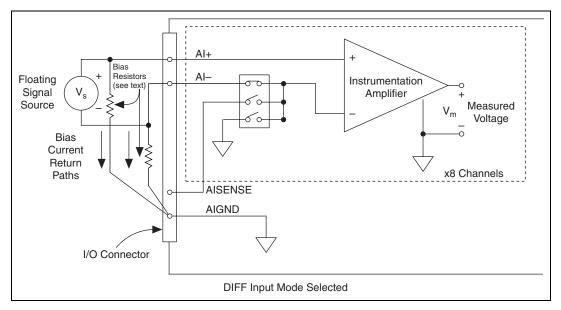
**Figure 2-6.** Differential Input Connections for Nonreferenced Signals
